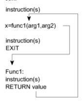
Functions may be **internal** and designated by a label, or **external** and designated by the data set member name that contains the function. The previous example illustrates an internal function named "func1".
