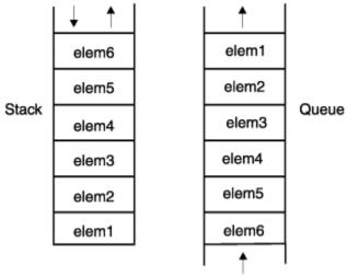
As shown in the following figure, the data stack that REXX uses combines the techniques used in adding elements to stacks and queues. Elements can be placed on the top or the bottom of a data stack. Removal of elements from the data stack, however, occurs from the top of the stack only.
