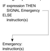
SIGNAL is useful for testing execs or to provide an emergency course of action. It should not be used as a convenient way to move from one place in an exec to another. SIGNAL does not provide a way to return as does the CALL instruction described in "CALL/RETURN Instructions" on page 54.
