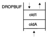
To drop a specific buffer on the data stack and all buffers created after it, issue the DROPBUF command with the number of the buffer. The first MAKEBUF creates buffer 1, the second creates buffer 2, and so on. For example, if an exec issued three MAKEBUF commands that created three buffers, when you issue DROPBUF 2, the second and third buffers and all elements within them are removed.
