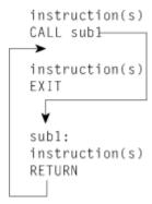
When calling an external subroutine, CALL passes control to the exec name that is specified after the CALL keyword. When the external subroutine completes, you can use the RETURN instruction to return to where you left off in the calling exec.
